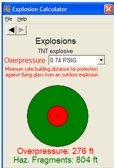
Figure 4 – Specifying the over-pressure level and results displayed
